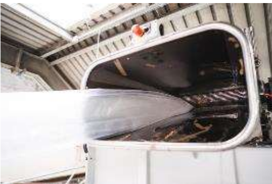
Photo 4: At the top, a feed roller at the hopper pulls the wound-on production waste from the roll into the shredding chamber.
