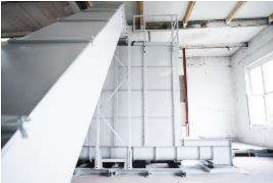
Photo 10: Since the shredder has a higher throughput than the two extruders, the shredded film is temporarily stored in a film silo to ensure continuous feeding.
