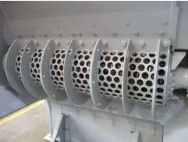
Image 3: The robust screen can be easily replaced to match different output particle sizes.
